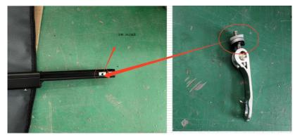
Slide rectangular screw plate into the AFK extension shaft. Screw in the Silver Adjusters with the bushes but only lightly, so it can be adjusted later on.
