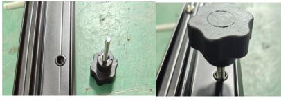
Fit the black tightening knobs into the available screw holes, but keep them loose so the flap plate can be removed and adjusted later on.
