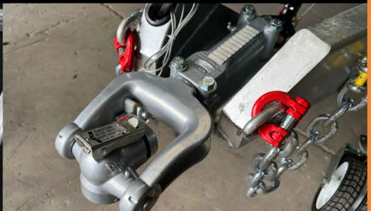
Full Off-road Coupling. Double ADR approved rated safety chains. Dual rear recovery points. Ark XO 750 Series extra heavy duty swing away dual wheel jockey wheel.
