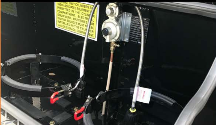
Completely plumbed from gas bottles to kitchen with dual bottle change over valve and gas certification certificate. Additional bayonet gas connection at rear of camper for a BBQ gas supply.
