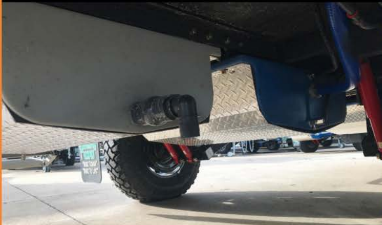
Water storage: 2 x 120L Freshwater water tanks and 1 x 80L plumbed grey water tank and system. 12.5L per min 12V Electric Pump. Water tank guards, water gauge.
