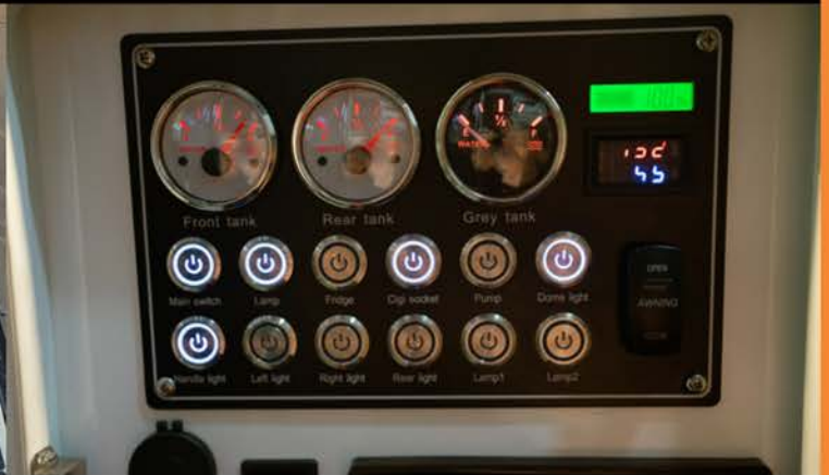
Control panel with water level gauges, multimedia system.
