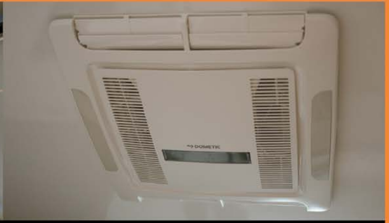
Roof Mounted Air conditioner.
