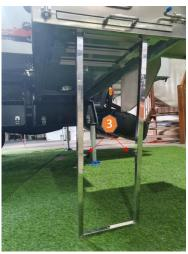
The kitchen can free stand however it is not recommended to do this whilst cooking as the extra weight of pots and food can put strain onto the slide runners over time. By ensuring that your kitchen is level will aid with the draining of the sink and will help your food cook evenly.
