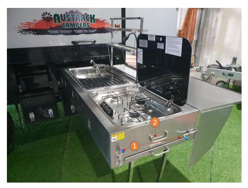
Once the kitchen is fully extended it is now time to lower the support legs, on the underneath of the kitchen there is a latch mechanism, press the small silver button to release the latch. This will allow the support legs to be lowered ready to support the kitchen slide.
