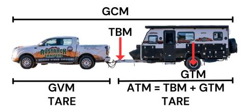
**GCM** Gross Combination Mass. The weight of your fully loaded vehicle and fully loaded trailer when hitched together.
