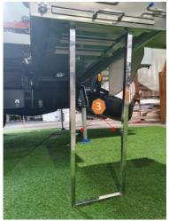
The kitchen can free stand however it is not recommended to do this whilst cooking as the extra weight of pots and food can put strain onto the slide runners over time. By ensuring that your kitchen is level will aid with the draining of the sink and will help your food cook evenly.
