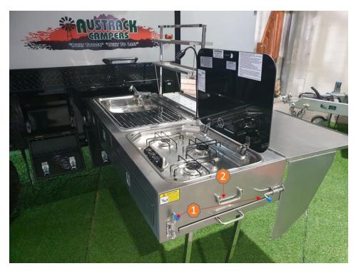
Once the kitchen is fully extended it is now time to lower the support legs, on the underneath of the kitchen there is a latch mechanism, press the small silver button to release the latch. This will allow the support legs to be lowered ready to support the kitchen slide.
