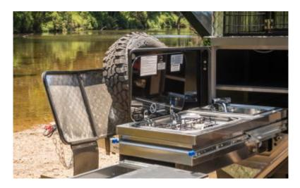
The kitchen is located at the front passenger side of the camper and can be accessed by opening the access hatch, once the hatch is open you will see 2 blue handles, one on each side, press down and gently slide the kitchen out.
