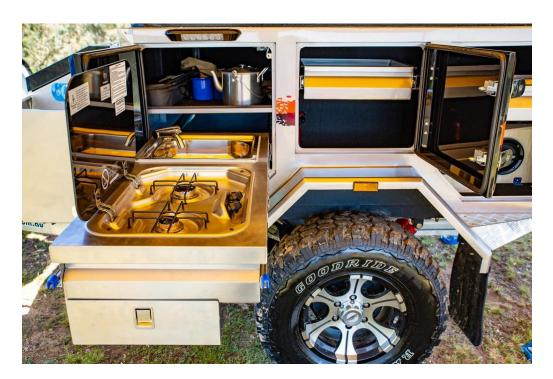
You will need to drop the sink waste hose out from the cutout in the bottom of the kitchen and runs this into a container to catch the water. Do not pour boiling water down the sink, the drain hose underneath is made of plastic, and it will melt with boiling water.
